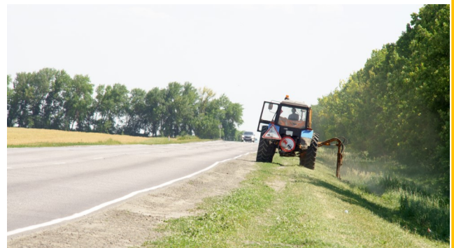
A shadow vehicle is not required when the mower works entirely from the shoulder or outside the travel lane.
